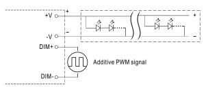
"DO NOT connect "DIM- to -V"
