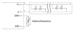
"DO NOT connect "DIM- to -V"
