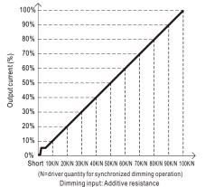
Note: 1. Min. dimming level is about 5% and the output current is not defined when 0% < Iout < 5%.
