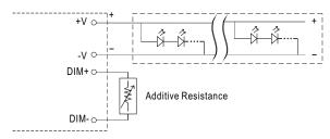
"DO NOT connect "DIM- to -V"
